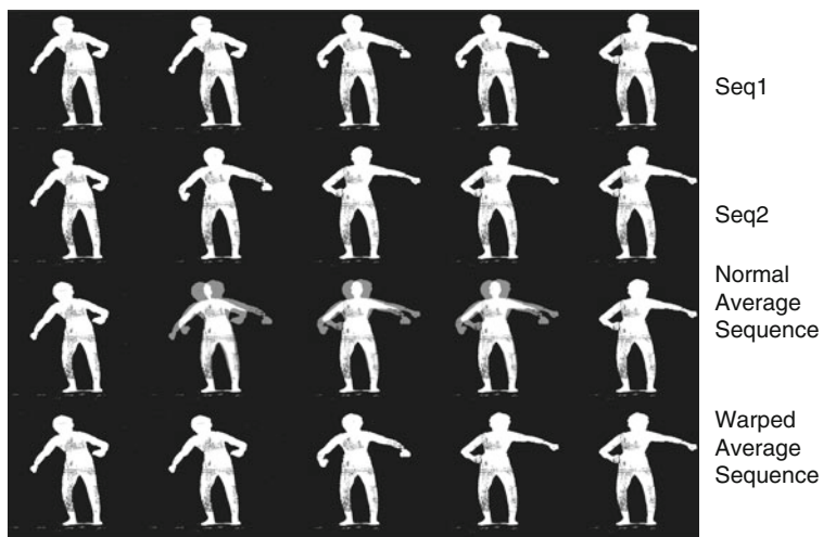
(R) Two sequences with differing rates of executions and their normal and warped average sequences.
