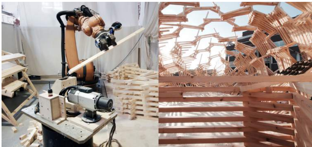
Figure 6 Left: robotic fabrication process. Right: DUO's inner view. © Andrea Quartara
