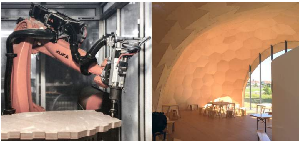
Figure 2 Left: robot milling from the public information panels. Right: internal view of the plate outlines that visually reflect the changing of Gaussian curvature. © Miro Bannwart
