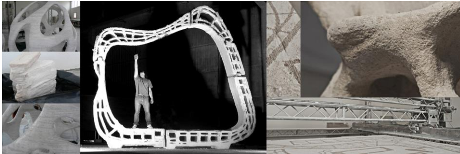
Figure 2. Material deposition 3d printing «D-shape 3d printing»
