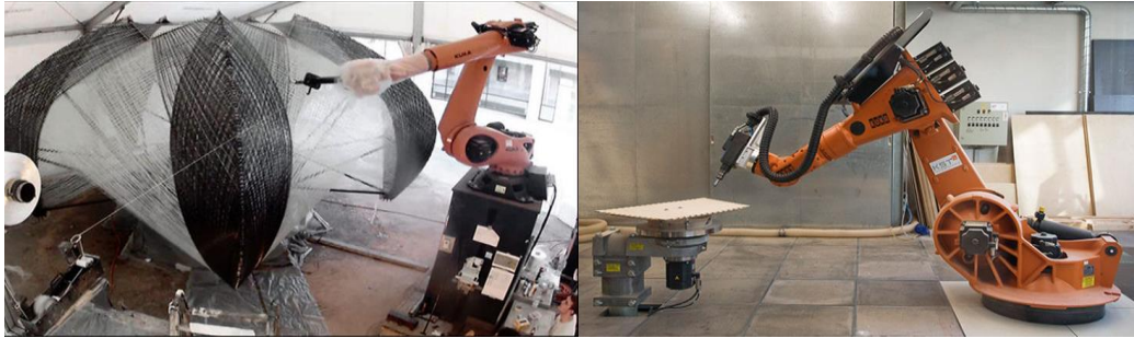
Figure 1. Robotic fabrication printing «ICD/ITECH research pavilion 2012»
