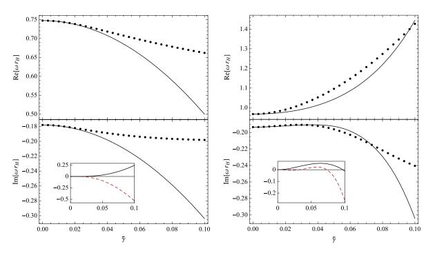
FIG. 3. Fundamental axial  $\ell = 2$  QNM frequencies of Schwarzschild BHs in dCS gravity as function of  $\bar{\gamma}$  for the tensor-led (left) and scalar-led (right) modes. Solid lines refer to Eqs. (33) and (34); bullets were computed through a direct integration method. The inset shows the relative difference between the two calculations for the real (solid black lines) and imaginary (dashed red lines) part of the modes.
