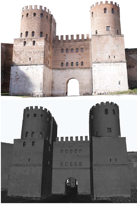
Fig. 5. Point clouds on the outside gate obtained through photogrammetry and SfM (top) and range sensor (bottom).
