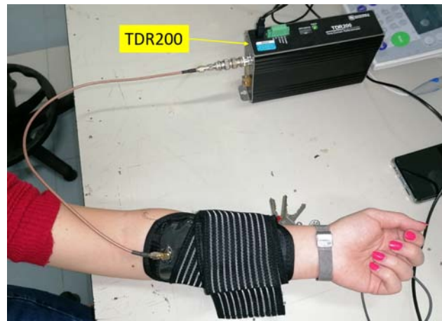
Figure 8. Picture of the experimental setup for measurements on human skin.
