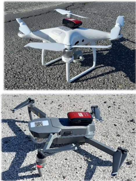
Fig. 3. Picture of the drone used as cooperative target: (a) DJI Phantom 4 Pro; (b) DJI Mavic Pro.
