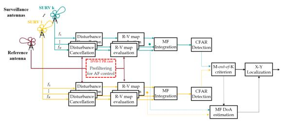
Figure 2. Developed AULOS® processing scheme.
