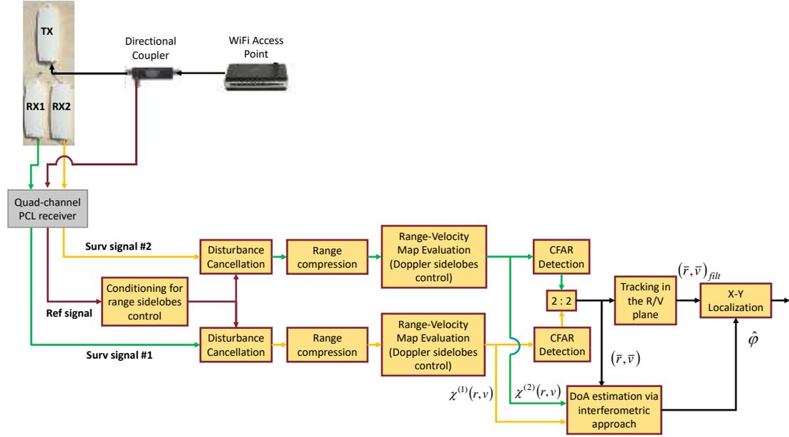
Figure 2 – WiFi-based PCL receiver set-up and signal processing scheme.
