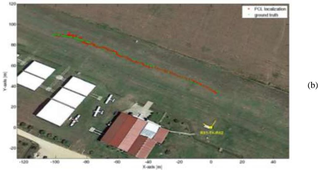
Figure 3. Test against a landing aircraft: (a) picture of the performed test; (b) PCL results compared to the available ground-truth.
