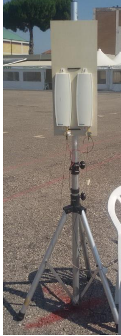
Figure 3.5. ANT24-1200: displaced configuration for a couple of antennas ('NODE 1').
