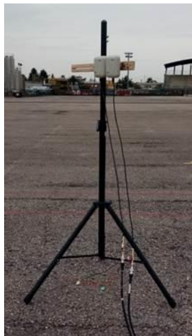
Figure 3.8. TL-ANT2409A: displaced configuration for a couple of antennas ('NODE 1').
