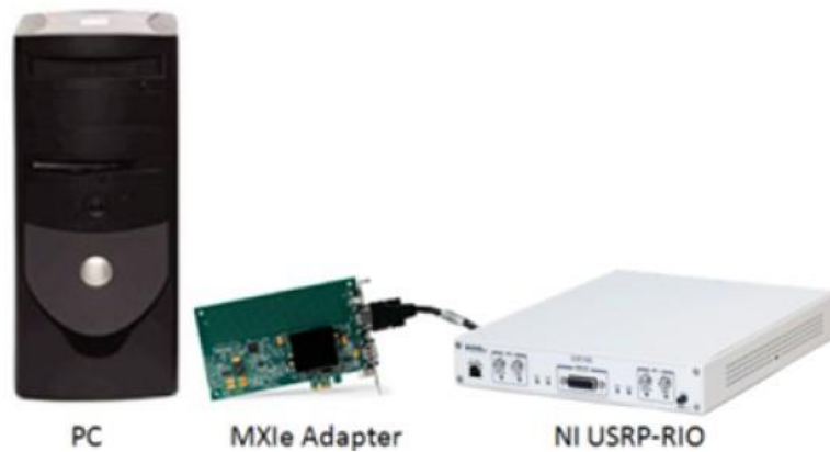
Figure 3.10. NI USRP-2955: URSP RIO system components.
