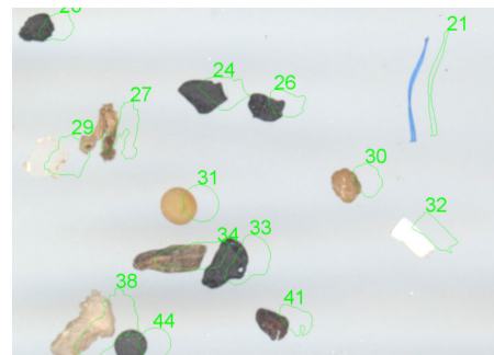
FIGURE 7. Detail of misaligned color image.
