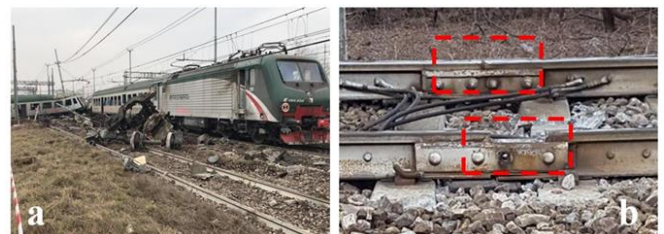
Figure 1. Pioltello (Mi, Italy). (a) Train accident; (b) Rail point where the failure may have occurred [2, 3]
