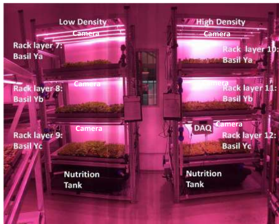
(a) Growth racks inside Agricola Moderna laboratory. Racks 7–9 are for the low density plants distribution, while Racks 10–12 are for high density plants distribution.
