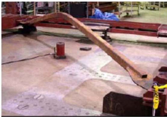
Traditional brace, buckled in compression
