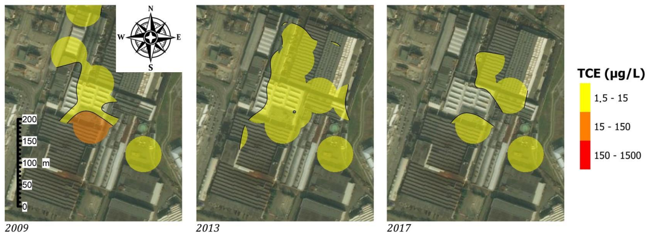
Figure 41. Contour maps representing the contamination state evolution of trichloroethylene (TCE) in the historical piezometric network (Ciampi et al., 2019 a ).
