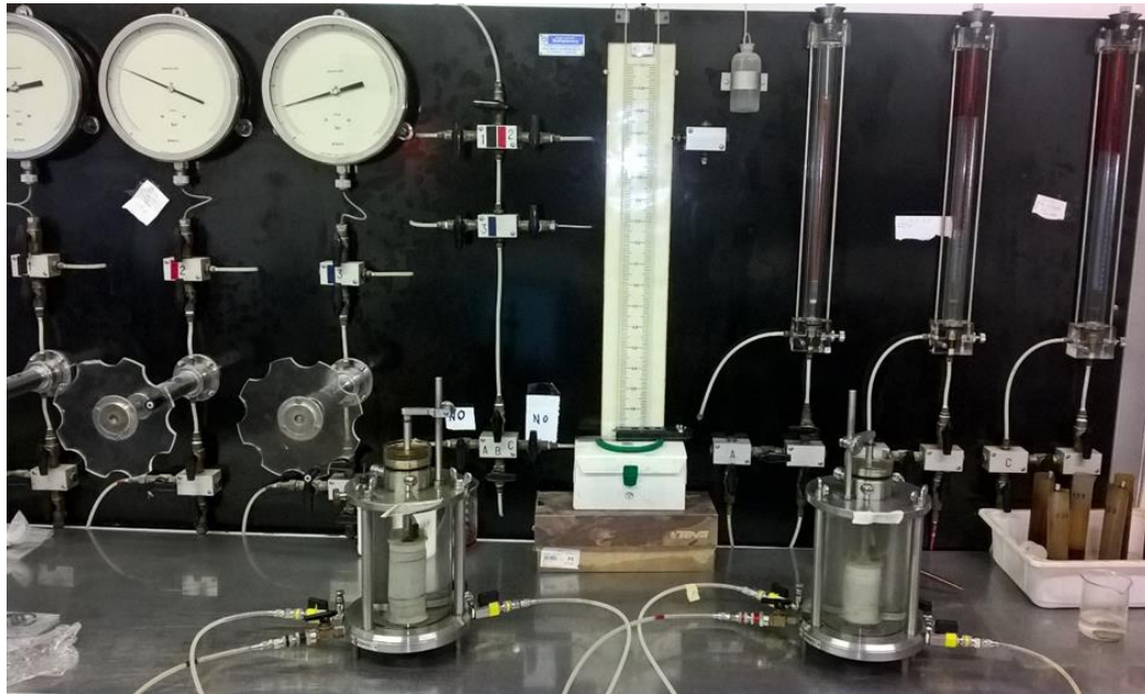
Figure 10. Instrumentation used for the determination of permeability in a triaxial cell.
