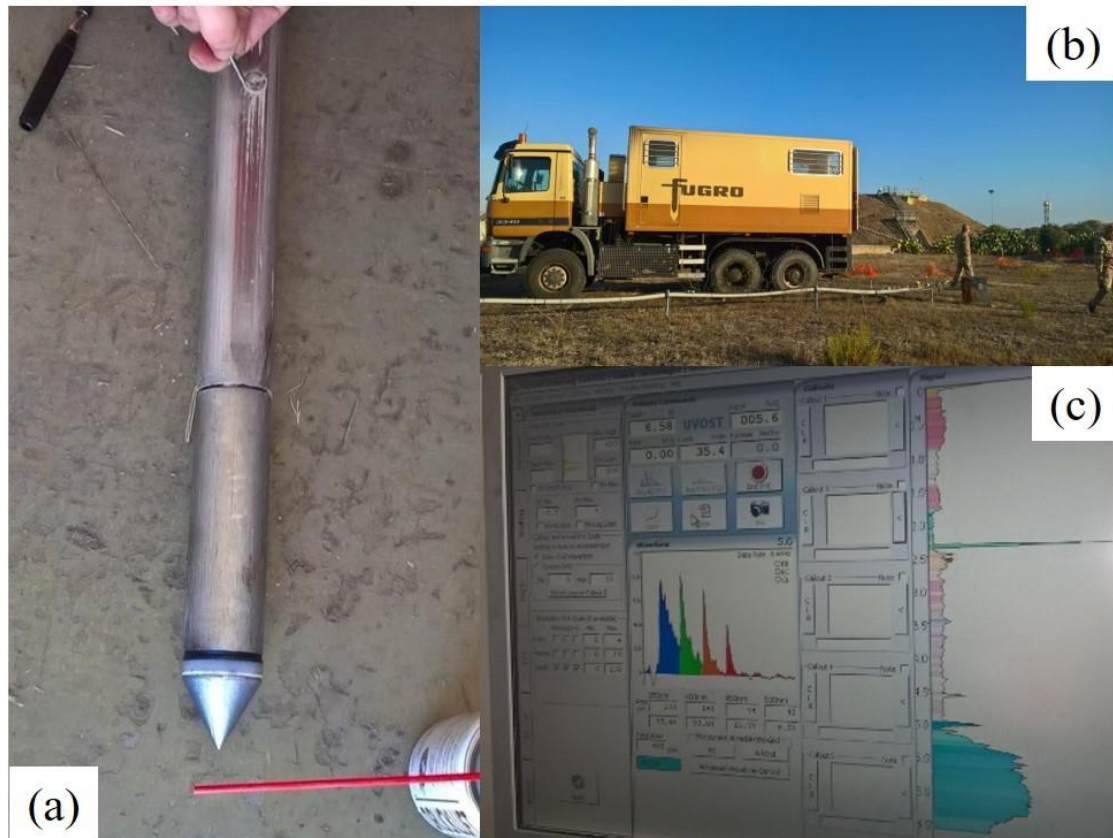
Figure 8. Conical tip adopted to realize the LIF profiles (a), truck used to transport the equipment inside the air base, fluorescence signal acquired in real time.
