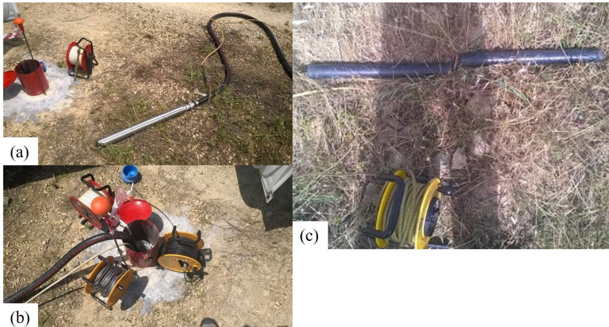
Figure 7. Instrumentation used for pumping tests (a, b) and slug tests (c).
