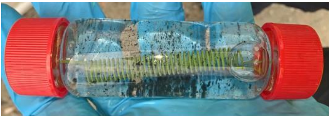
Figure 54. Evidence of the PlumeStop® distribution inside the intermediate aquifer.
