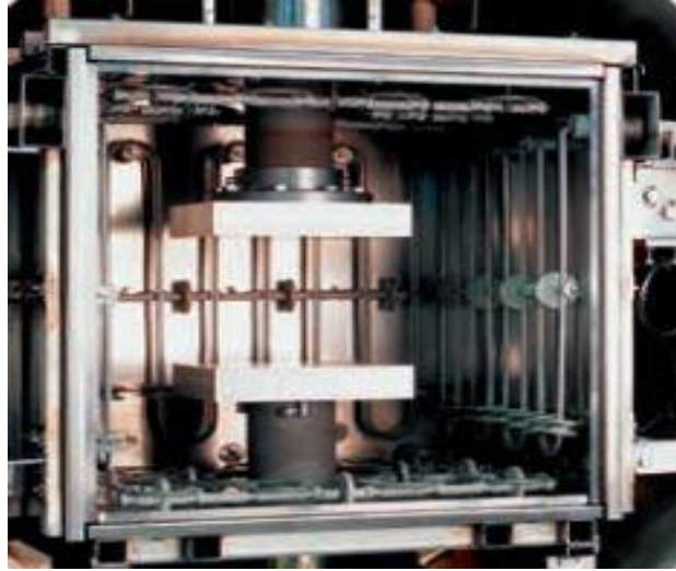
Figure 7. The diffusion bonding resistance heated
