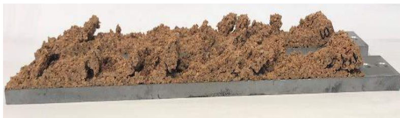
Figure 20. NL10 intergranular fracture after shear test.
