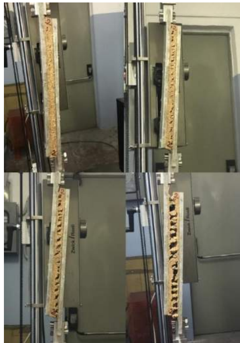
Figure 19. Crack propagation during NL25 shear test.
