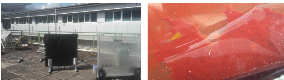
Figure 5.4 single-stage 60 L flat plate out-door photo fermentation
