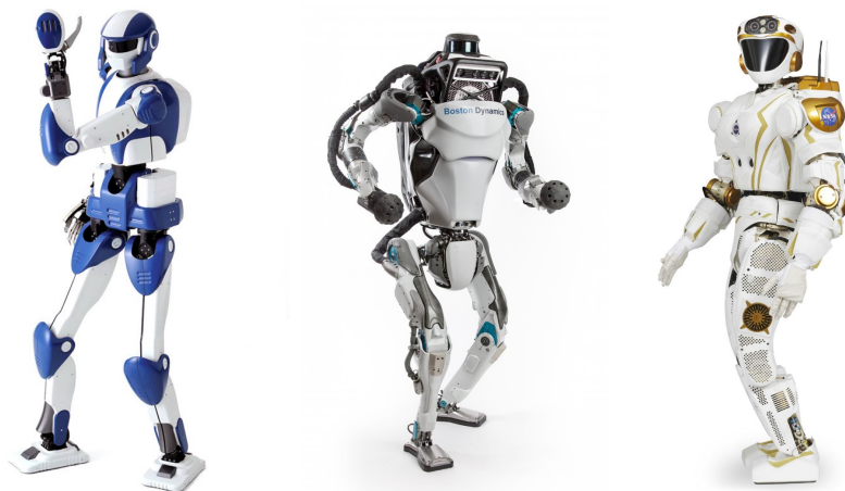
Figure 1.2. Modern humanoid robots: HRP-4 from Kawada Robotics, Atlas from Boston Dynamics and Valkyrie from NASA.
