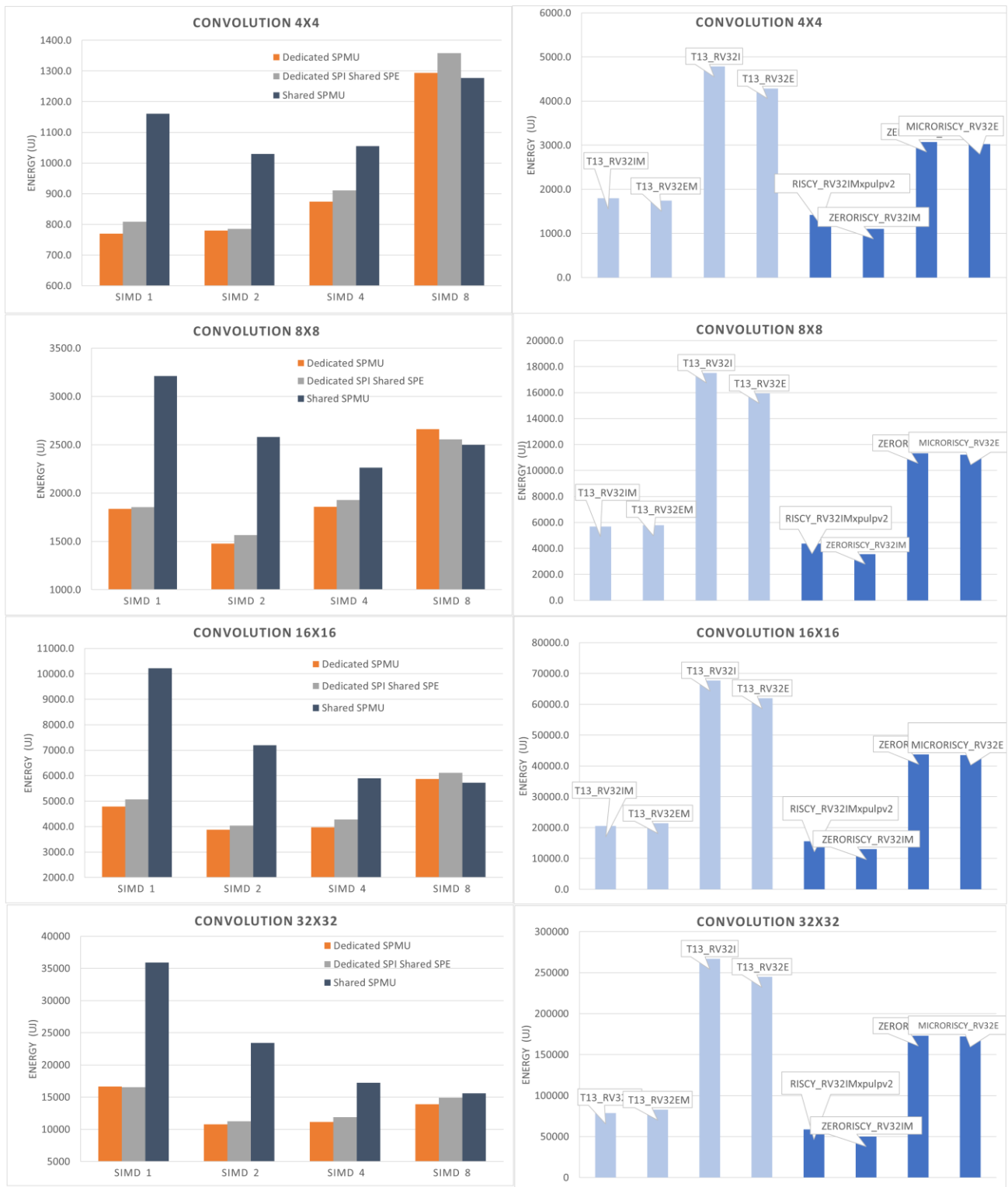
Figure.5.20. Energy Consumption for running each implementation at the top frequency on the different convolution sizes
