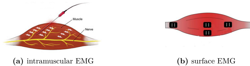
Figure 2.1. Schematic example of the techniques used to acquire EMG signals. In (a) EMG is recorded using an invasive method, with needles that record localized information within the muscles. In (b) the global muscle activity is recorded via surface electrodes placed on the skin.
