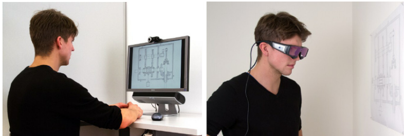
Figure 2.8. Remote (left) and head mounted (right) infrared camera based eye tracking systems. In the first case the device is placed under the display monitor, in the second case it is embedded in the glasses worn by the user. Figure credit: Lohmeyer et al. 2013.
