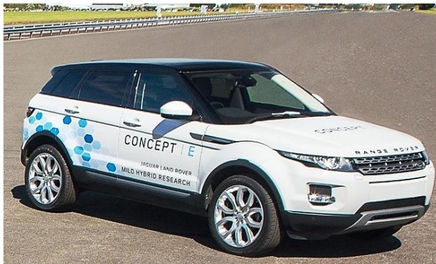
Figure 1 The carbon/flax hybrid composite roof produced for the Range Rover Evoque. This hybrid structure has been developed within the CARBIO project which involves Jaguar Land Rover, Composites Evolution, SHD Composite Materials, KS Composites, Delta Motorsport and Cranfield University [Vijayenthiran, 2015; Caliendo, 2016].
