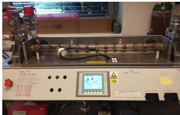
Figure IV. 3 The PECVD reactor used.
