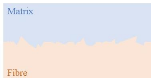
Figure I. 5 Interface bonds formed by mechanical interlocking.
