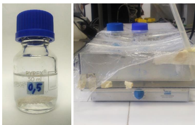
Figure IV. 1 An example of flax fabric inside the lab jar and the thermostated water bath system used during the treatment.
