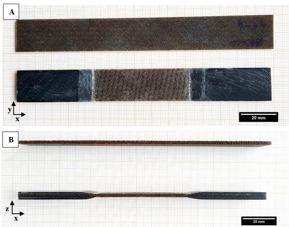
Figure II. 19 Example of flax/epoxy composite specimens without and with the presence of the glass fibre/epoxy tabs on the y-x plane (A) and on the z-x plane (B).
