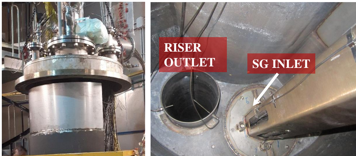
Fig. 2-7 – External and internal view of the Separator
