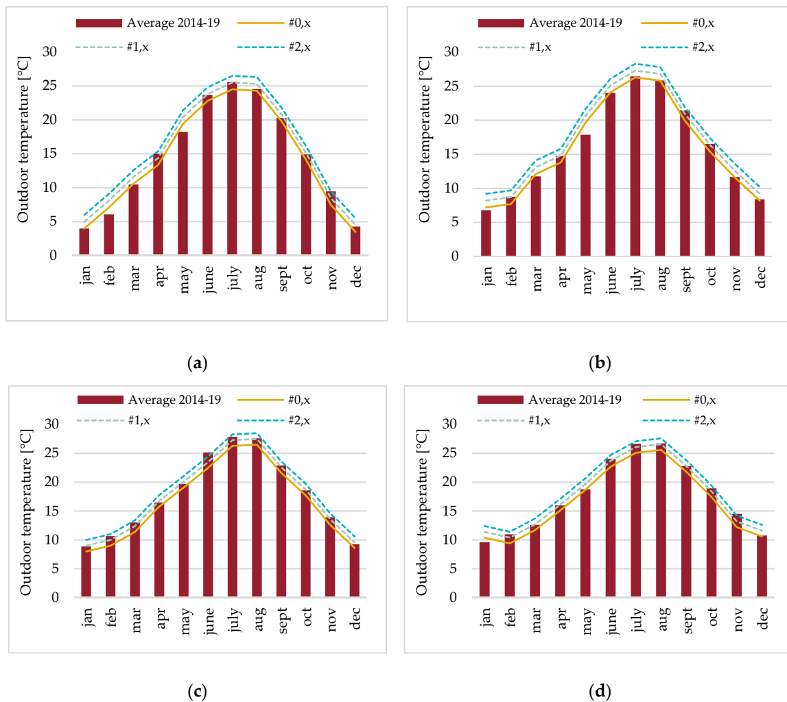
Figure 2. Comparison between simulated data and the climate average data related to years 2014–2019; (a) Milan; (b) Florence; (c) Rome; (d) Naples.
