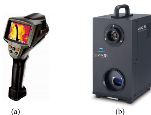
Figure 1. (a) Thermal camera Testo 882. (b) Laser scanner Konica Minolta Vivid 9i.
