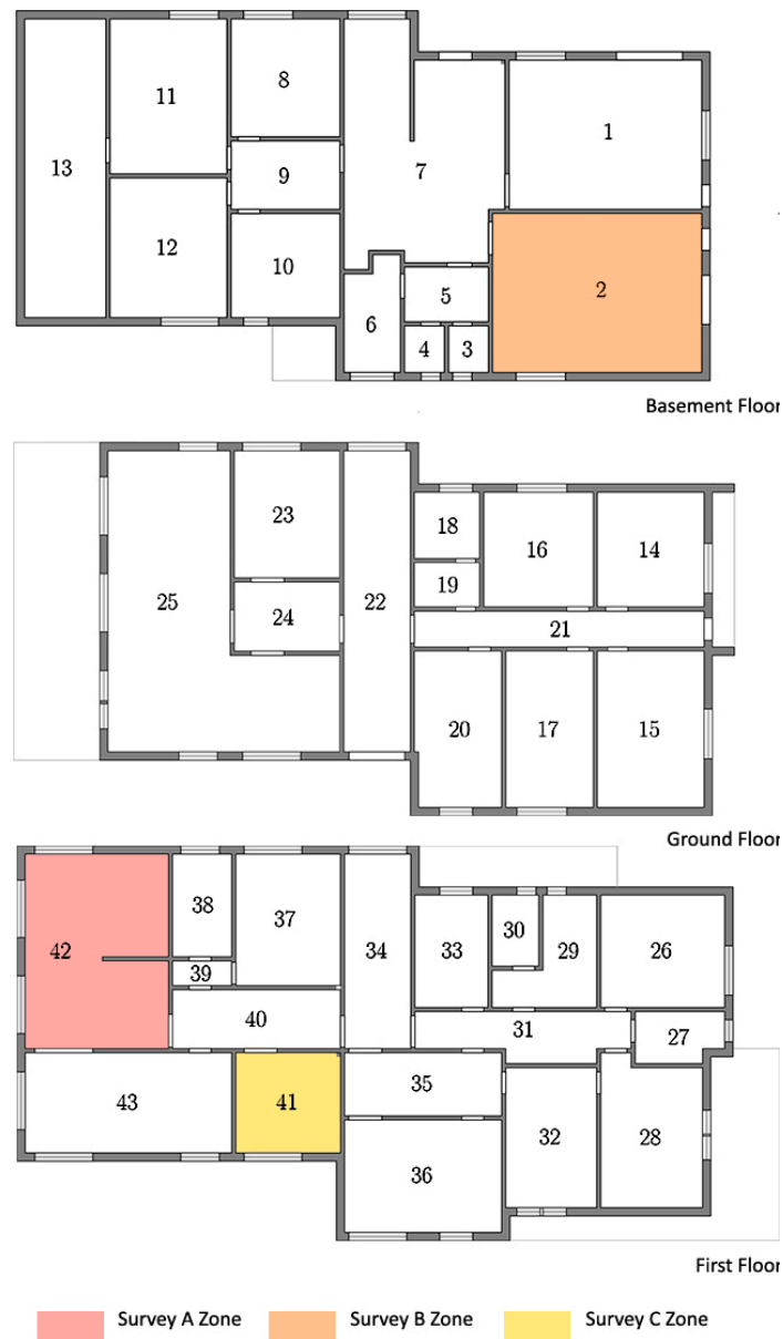
Figure 6. Thermal zones. The highlighted zones refer to the rooms where the monitoring surveys were carried out.
