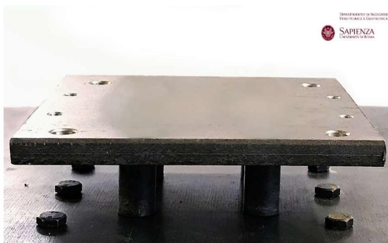
Figura 9. 1 Hysteretic Vibration Absorber – Rubber (HVA-R)
