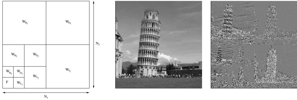
Figure 3.6. Example of wavelet transform computed over three scales on an image of size N_1 \times N_2 using an orthonormal basis. Left panel. Schematic decomposition of the image into its detail levels at all the three scales along the horizontal, vertical and diagonal directions, W_H , W_V and W_A , respectively. The approximation level is denoted as F , and it is obtained from the low-pass filtering. Middle panel. Original image. Right panel. Maps of the wavelet coefficients according to the same scheme as in the left panel [taken from 65].
