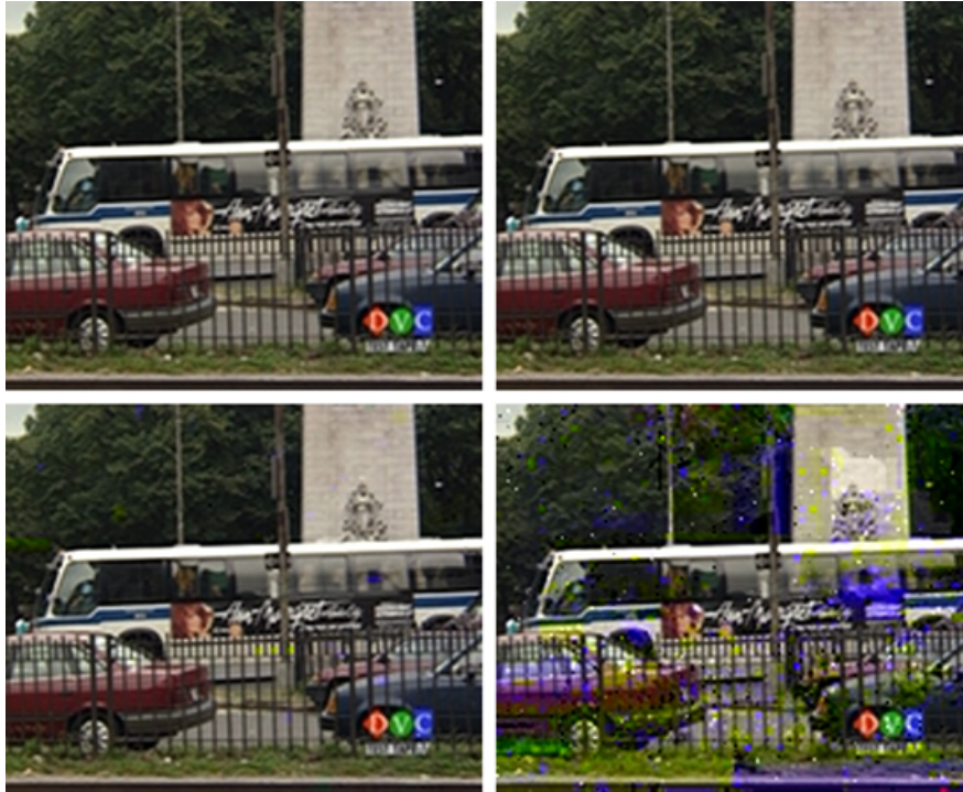
FIGURE 5.9: x264, output frame coded with exact (top left) and approximate SRAM (0xFFFFFFFF looseness mask), fault rate 10^{-6} (top right), 10^{-4} (bottom left) and 10^{-2} (bottom right) [errors/access].
