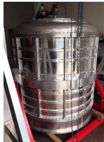
(c) Cryostat external shell.
