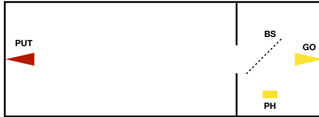
Figure 3.6: Sketch of the room temperature setup. Black lines correspond to the eccosorb panels of the anechoic chamber. The pixel under testing (PUT) is illuminated by a modulated Gunn oscillator (GO) and is located in the antenna far field. A beam splitter (BS) divides the emitted radiation and the power emitted by the Gunn is monitored by means of a millimetric diode (PH).
