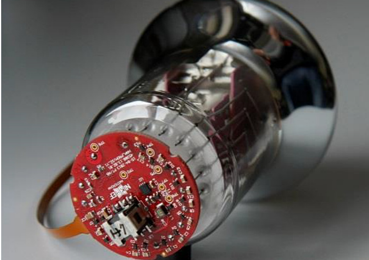
Fig 15: The PMT base board mounted on a 3-inch PMT.
