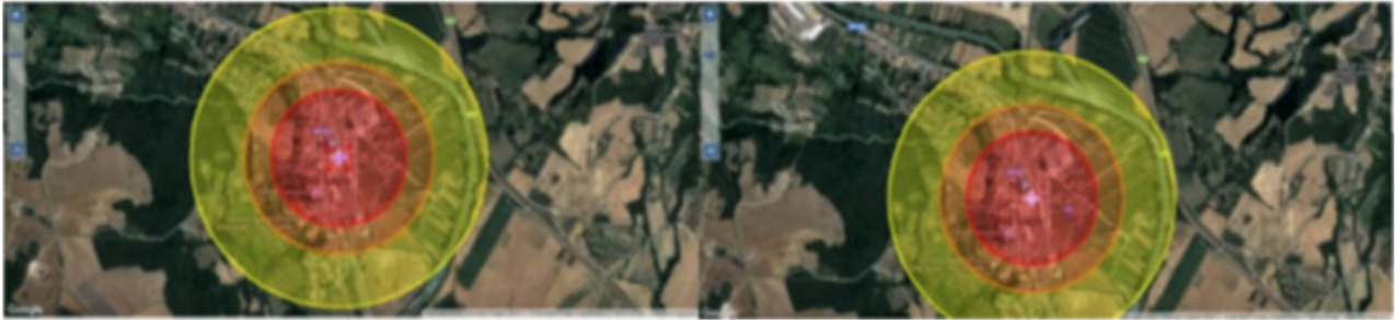
Fig. 8 Shock wave generated by detonation (left butane, right propane), different colors with different intensity, from the highest (red) to the lowest (yellow).
