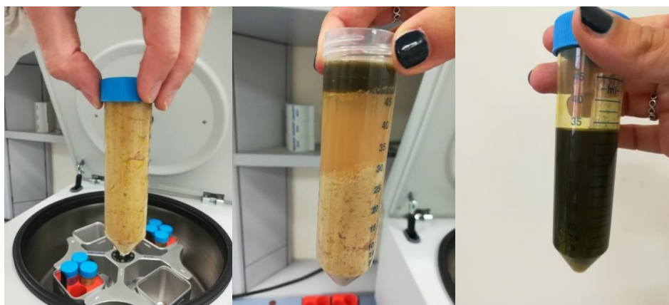
Fig. 3.12: Stages of oil extraction from olives. Left image, the olive paste is poured into the Falcon to be inserted in the centrifuge. Central image, we note the stratification obtained after centrifugation, oil as supernatant, vegetation water in the middle, pomace and hazels in the bottom. Right image, the supernatant oil of the various extractions of the same olive sample is collected in a Falcon.
