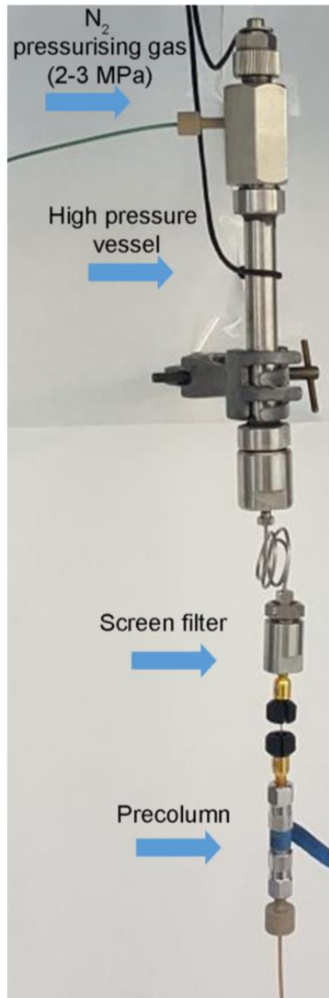
Figure 25 Image of the capture system
