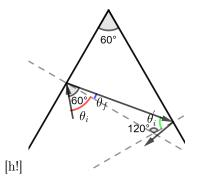
Figure 4: Relation between the incident angles of two subsequent bounces. The figure shows that the initial condition  $\theta_i + \theta_f = 60^\circ$  implies  $\theta_i = \theta'_i$ , in fact  $\theta'_i = 180^\circ - 120^\circ - \theta_f = 180^\circ - 120^\circ - (60^\circ - \theta_i) = \theta_i$ .
