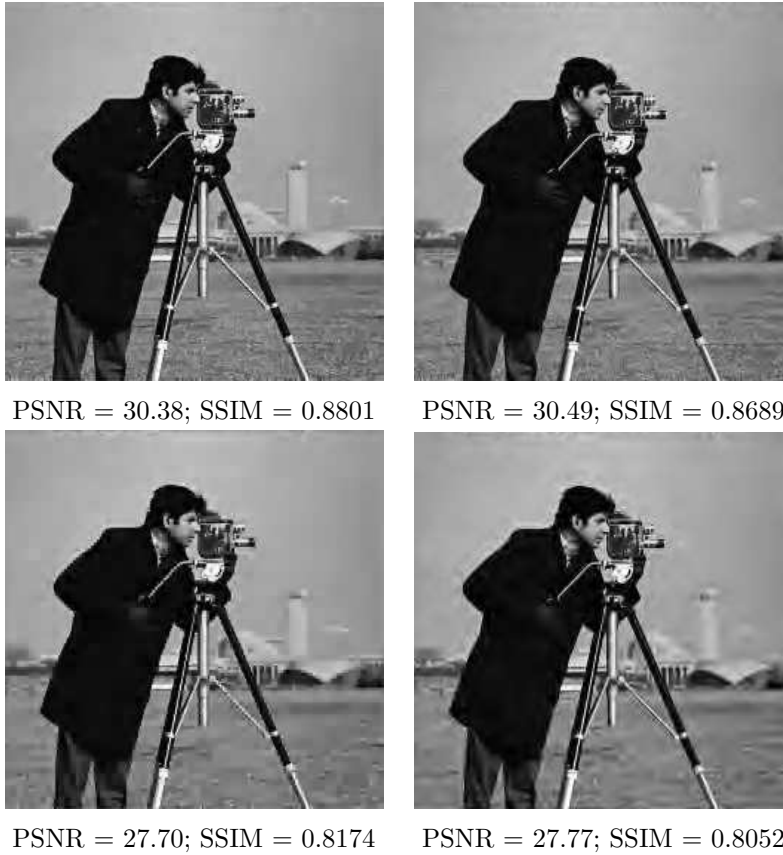
Figure 5: Compression tests on the Cameraman image. Top ) SPIHT compressed image at bpp = 0.5 using: the nonstationary filters having N = 1 , \tilde{N} = 3 , \mu = 0.1 and L = 8 ( left ) and JP2K-like stationary biorthogonal filters ( right ). Bottom ) SPIHT compressed image at bpp = 0.3 using: the nonstationary filters having N = 1 , \tilde{N} = 3 , \mu = 0.1 and L = 8 ( left ) and JP2K-like stationary biorthogonal filters ( right ).
