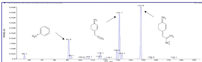
**Figure IV.1A.** Product ion scan spectrum obtained for *Cis*-4,4'-DMAR at a collision energy of 25eV
