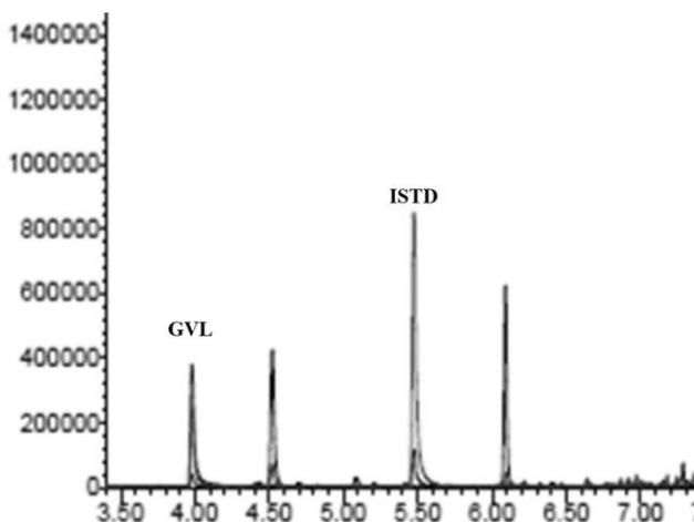
**Figure VI.3.** Extracted chromatogram of an urine sample with GC-MS operating in full scan mode.
