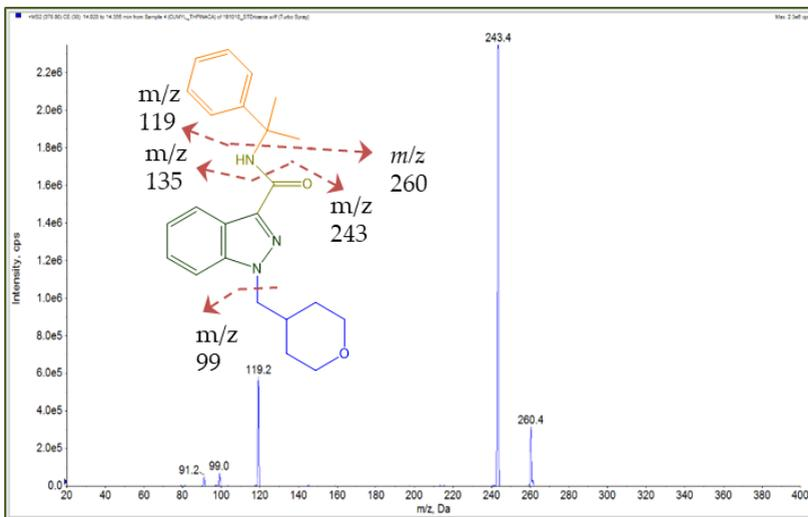
**Figure VII.3.** Product ion scan spectrum obtained for CUMYL-THIPINACA at a collision energy of 30eV
