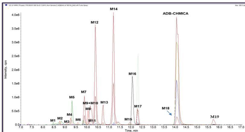
**Figure VII.4.** Extracted chromatogram with MRM mode (QqQ) of the same sample analysed with QTOF technique
