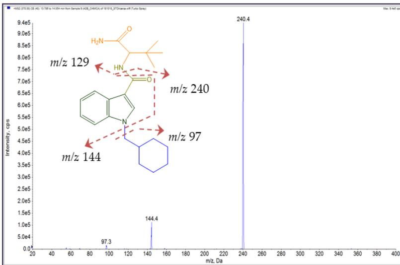
**Figure VII.2.** Product ion scan spectrum obtained for ADB-CHMICA at a collision energy of 30eV
