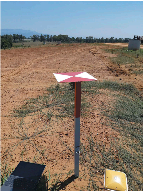
Figure 3. One of the photogrammetric markers.
