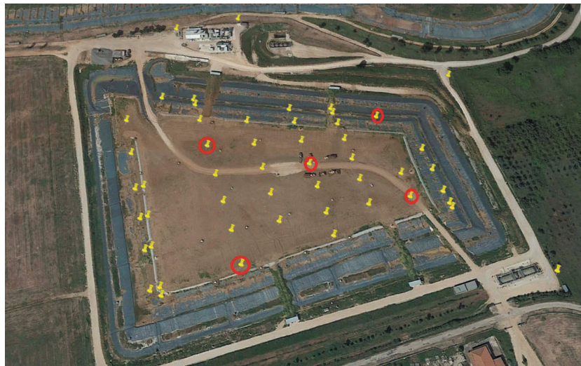
Figure 2. The study area with the surveyed point, CPs are in red circle.
