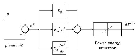
Figure 4. A second-level proportional-integral-derivative (PID) controller.
