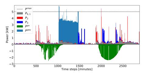
Figure 8. Scenario 1: Power consumption and injections within the node (data from [61]).
