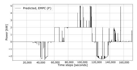
Figure 13. Scenario 3: Net node power profile resulting from the capacity tariff (data from [61]).
