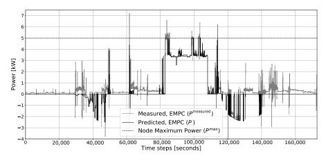
**Figure 10.** Scenario 2: Planned and real (measured) net node profile when only EMPC is enabled (data from [61]).
