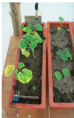
Figure 2. Pilot plant for the application of phyto-electroremediation (phyto-ER).
