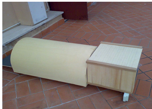
Figure 34 Scale model of tunnel and pre-tunnel.
