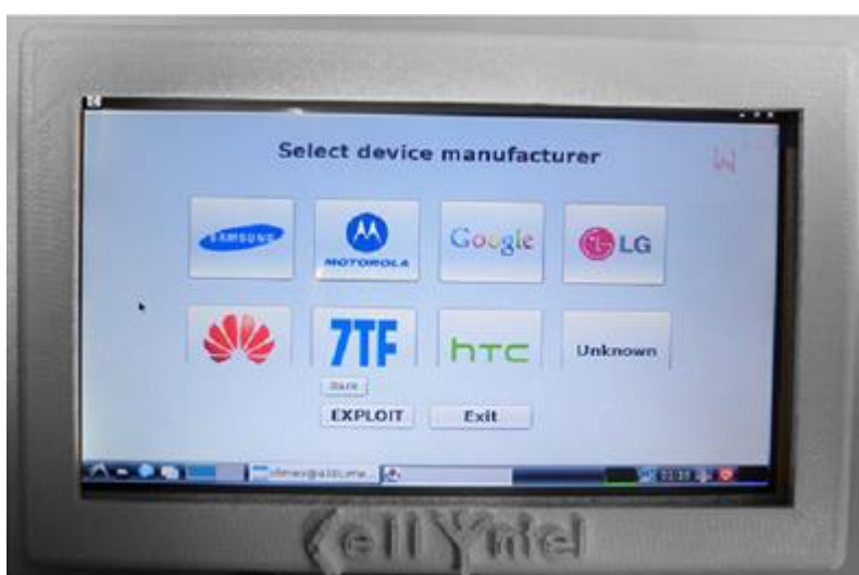
Figure 4. CellIntel assembled prototype in function: touch screen user interface during the choice of the device to be imaged.
