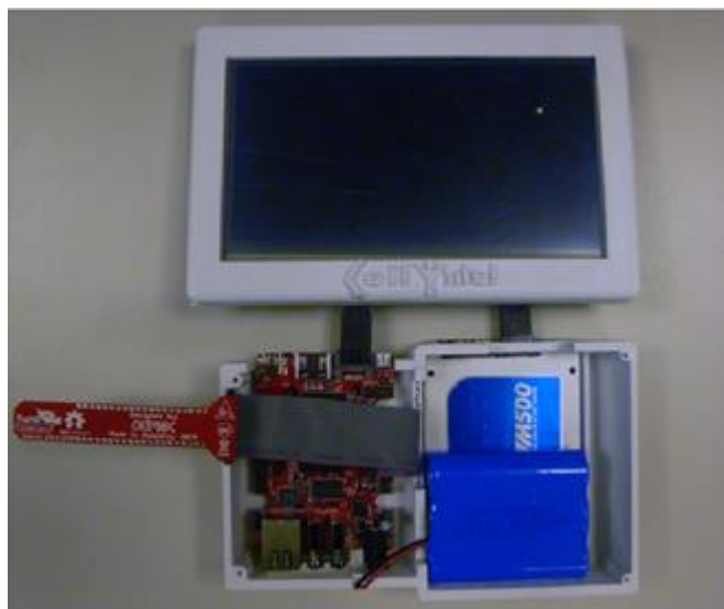
Figure 3. CellIntel prototype’s components during the manual assembly: LCD screen, 3D printed screen case, battery, SSD hard disk drive, printed circuit board, cables for connections among components and 3D printed base case.
