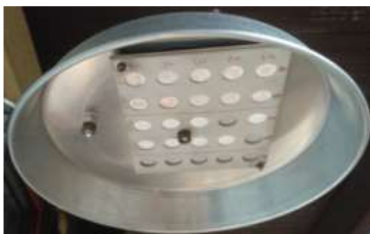
Figure 17 – Sample holder for outdoor environmental exposures.
