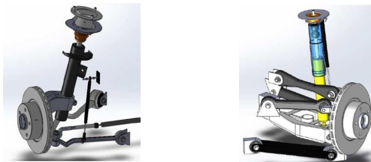
Figure 5: CAD of the original BMW front kinematic suspension at (left) and the rear one at (right).
