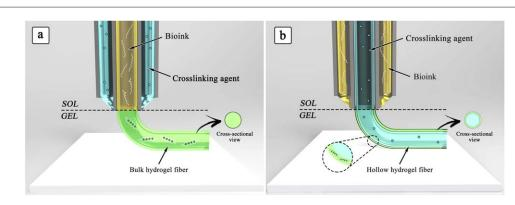
**Figure 2.** Schematics representation of a co-axial extruder: by inverting the deliver site of the bioink and crosslinking agent solution, either (a) bulk or (b) hollow hydrogel fibres can be laid down.
