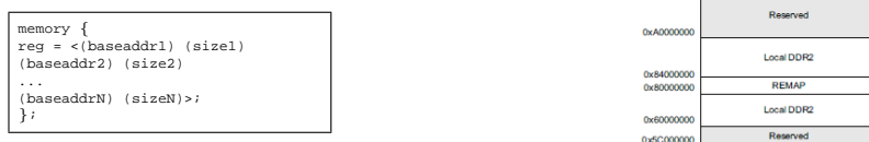
Fig. 1. On left: Memory node in device tree. On right: Vexpress Cortex A9 board memory map (extract)
