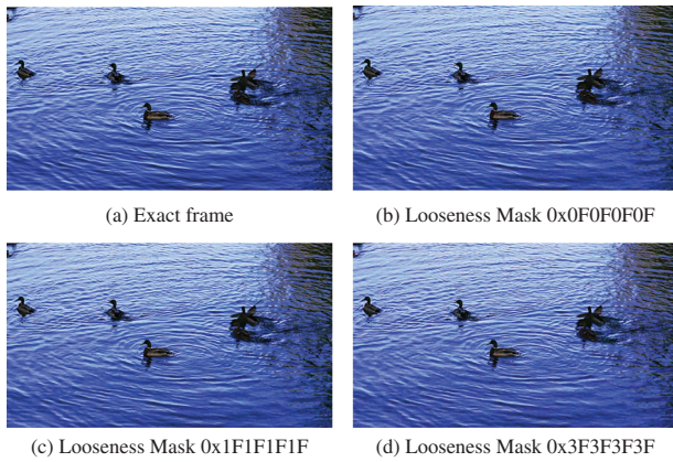
Fig. 5. \times 264 , output frame with different looseness levels and fault rate 10^{-4} [errors/(bit \times s)].
