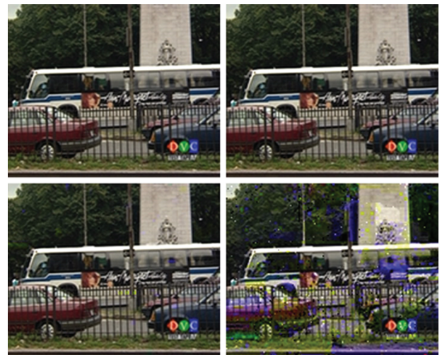
Fig. 7. \times 264 , output frame coded with exact (top left) and approximate SRAM ( 0 \times \text{FFFFFFF} looseness mask), fault rate 10^{-6} (top right), 10^{-4} (bottom left) and 10^{-2} (bottom right) [errors/access].
