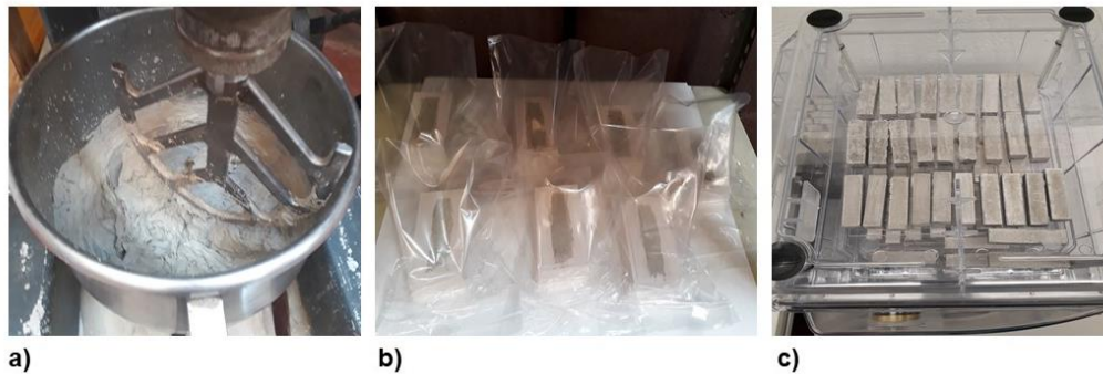
Figure 3. Mixing (a) and curing (b-c) of natural hydraulic lime-based mortars.
