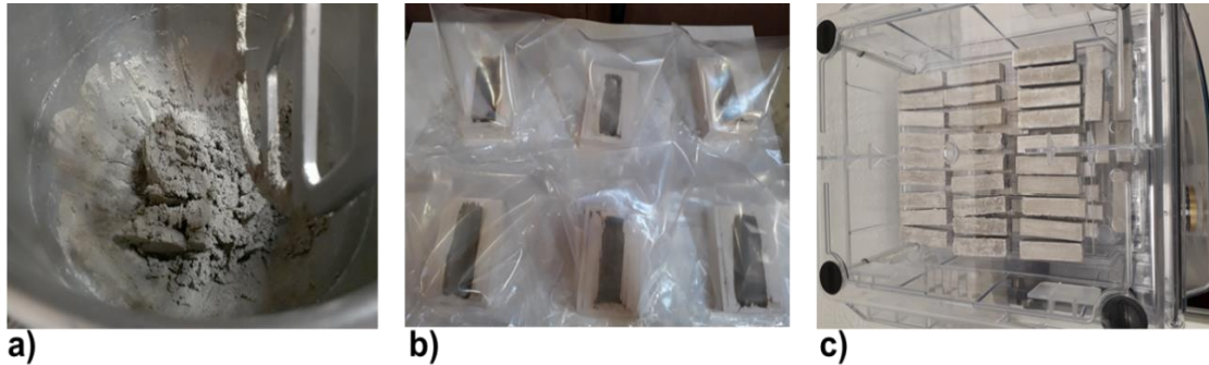
Figure 4. Mixing (a) and curing (b-c) of cement-based mortar samples.
