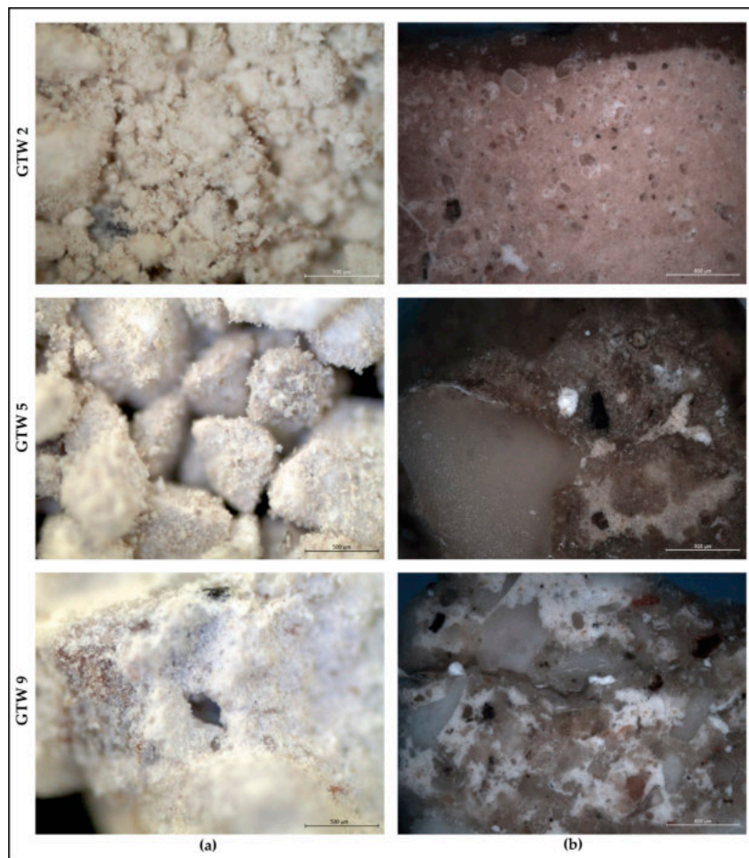
Figure 3. OM observation of mortar samples 2, 5, and 9, (a) direct mode and (b) polished sections. All observation was done in darkfield observation mode and 5× magnification.
