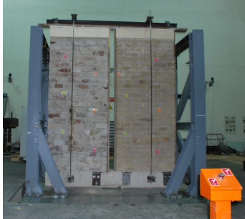
Figure 2 The real-scale mock-ups on the shaking table (see online version for colours)
